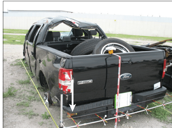
Figure 3: Arrow shows damage to Ford's back bumper from the impact with concrete traffic barrier (event 4)
