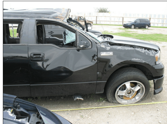
Figure 7: Damage from the rollover on the vehicle's right side and roof
