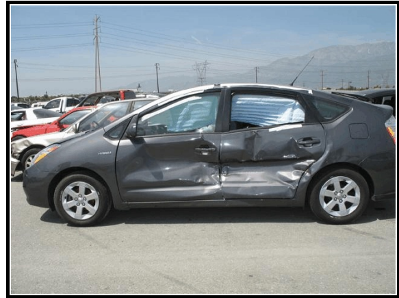
Figure 6. Left side damage
