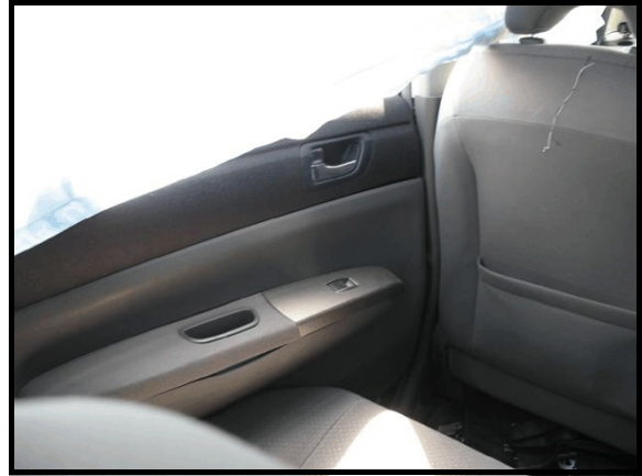
Figure 7. Left interior intrusion
