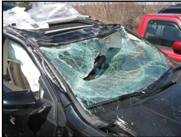
Figure 5: Ford roof deformation as a result of the rollover.
