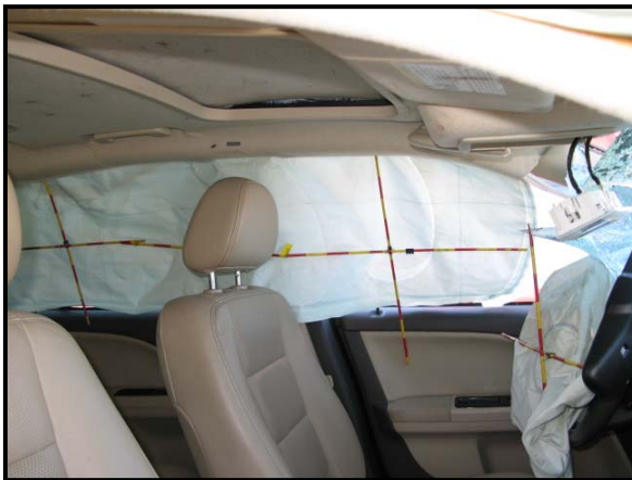
Figure 7: Deployed left curtain air bag.
