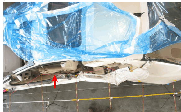
Figure 7: Top view of the Cadillac's left side crush profile represented by the string (arrow)
