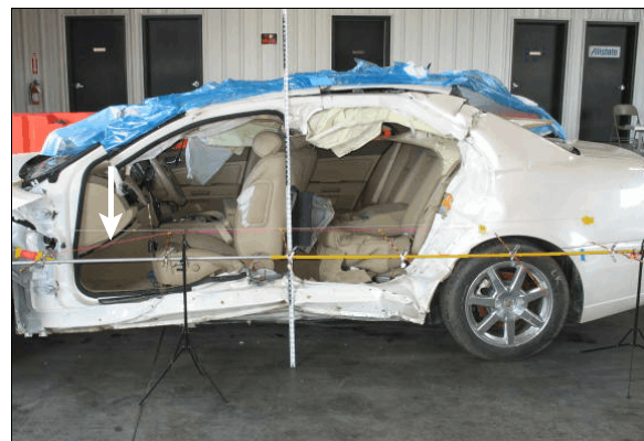
Figure 6: Arrow shows the string representing the crush on the Cadillac's left front and left rear doors
