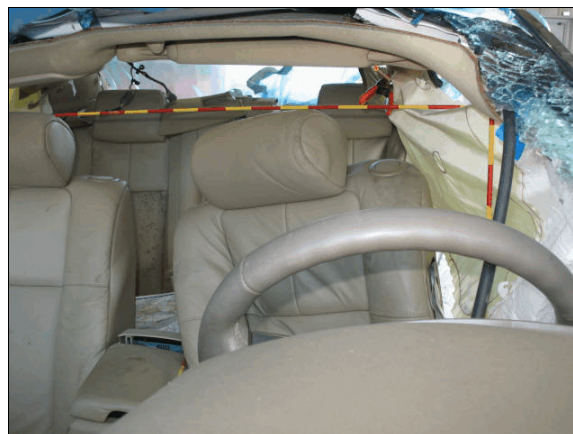
Figure 8: Lateral displacement of the driver's seat back
