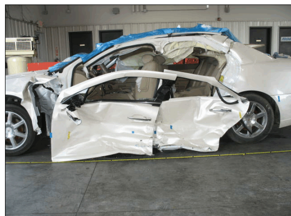
Figure 4: Damage to the left side plane of the Cadillac from the impact with the front of the Dodge
