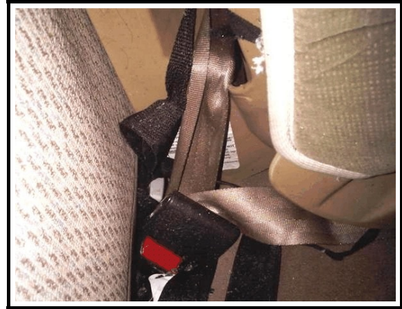
Figure 8. Second row center lap belt routed through CRS and buckled (Police photo)
