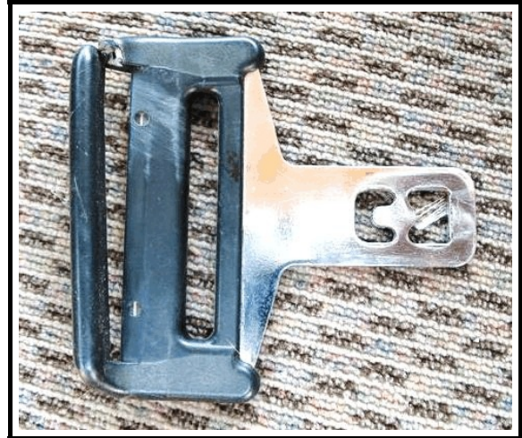
Figure 6. Driver's safety belt latch plate showing scuffs and fracture
