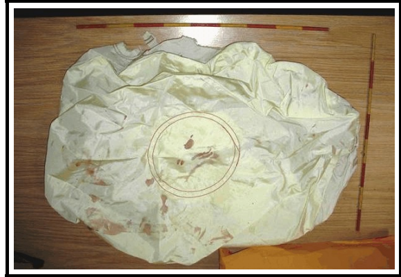
Figure 9. Driver's frontal air bag
