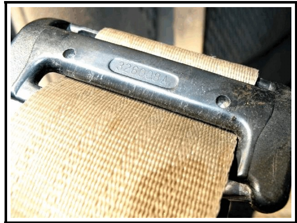
Figure 7. Front right occupant's latch plate showing loading marks
