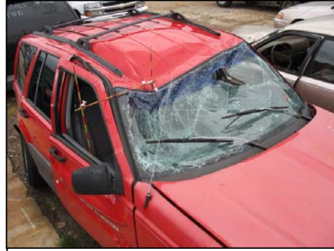
Figure 9: Rollover damage from above, right front
