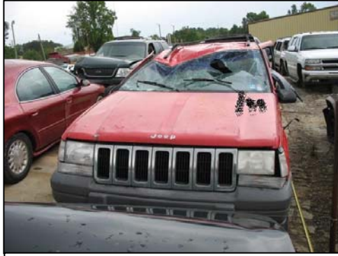
Figure 8: Rollover damage from front
