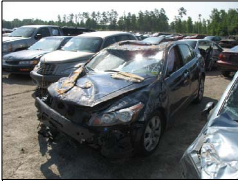
Figure 5: Rollover damage from front left
