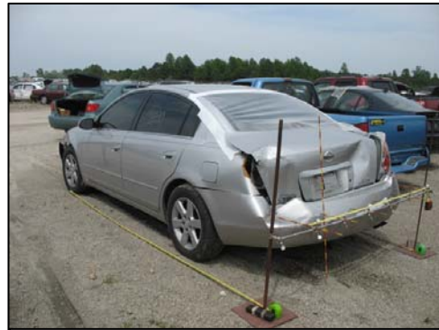
Figure 10: Back left view of the rear end damage.
