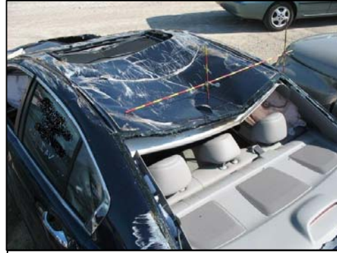
Figure 6: rollover damage from above, left rear
