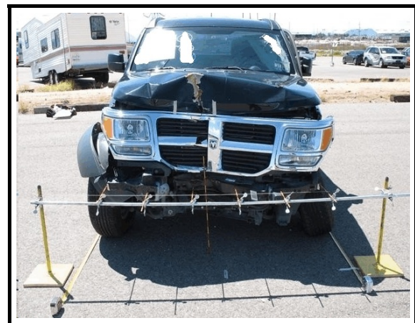
Figure 6. Dodge Nitro crush measurements, Event 3
