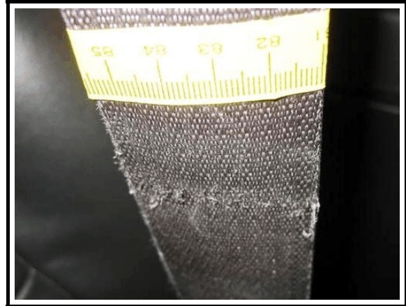
Figure 6. Front right occupant's safety belt webbing, 2008 Ford Escape
