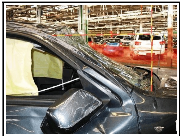
Figure 4. Maximum vertical crush measurement, 2008 Ford Escape
