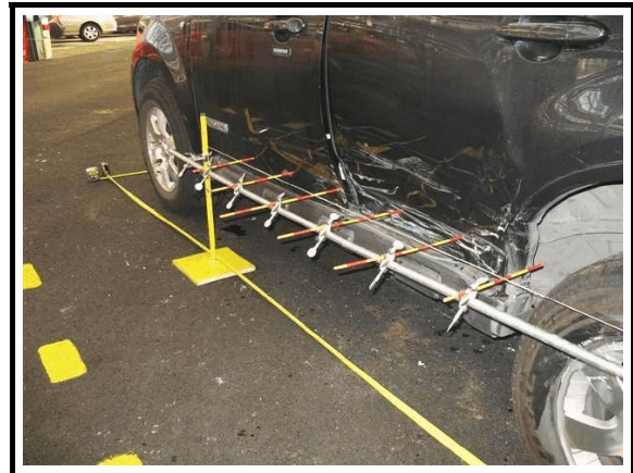
Figure 3. Left side crush profile, 2008 Ford Escape
