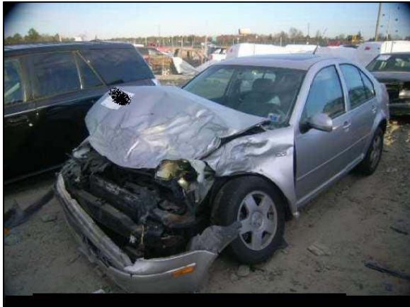
Figure 7: Impact damage to the Volkswagen from the front left.
