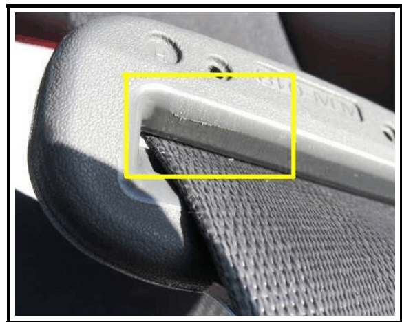
Figure 5. Scuff to safety belt latch plate resulting from occupant loading
