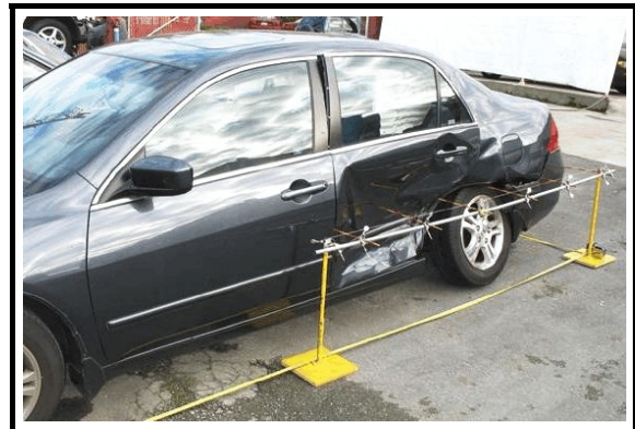
Figure 4. Subject vehicle showing left side crush profile measurement
