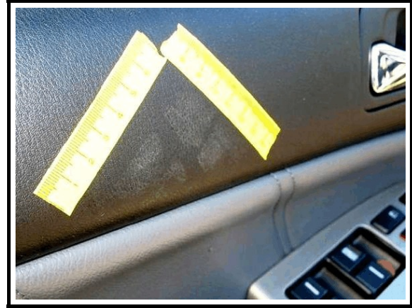
Figure 8. Scuff to door panel resulting from occupant loading
