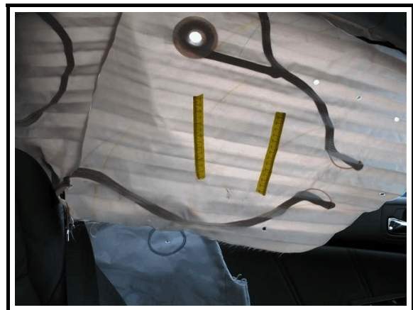
Figure 7. Location of hair and skin oil transfer on the left IC air bag
