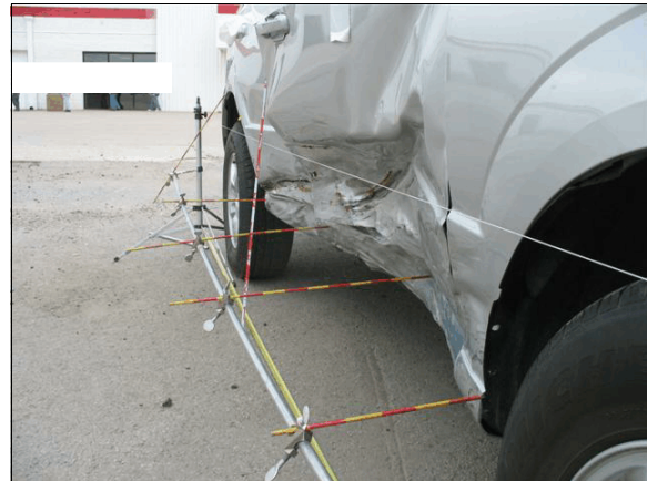
Figure 8: The maximum crush occurred on the sill
