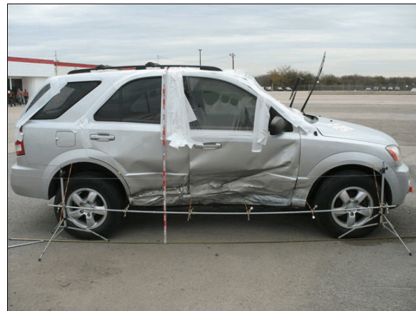
Figure 4: Damage on the right side plane of the Kia from impact with the front plane of the Ford
