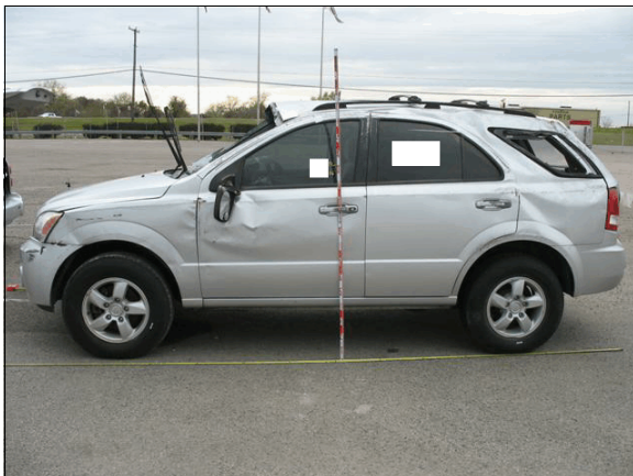
Figure 5: Damage on the left side plane of the Kia from the rollover
