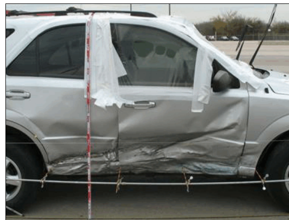
Figure 7: Damage on the right side plane of the Kia from the impact with the front plane of the Ford
