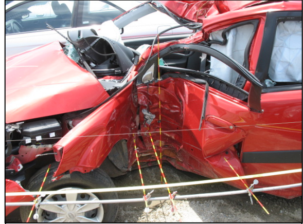
Figure 6: Lateral view of the pole impact damage.
