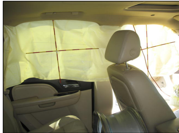
Figure 6: View of the left side forward IC air bag located in the first two seating rows
