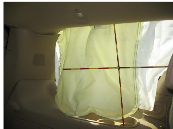
Figure 7: View of the left rearward IC airbag located in the third seating row
