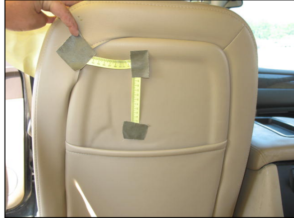
Figure 5: View of the contact point on the back of the driver seatback
