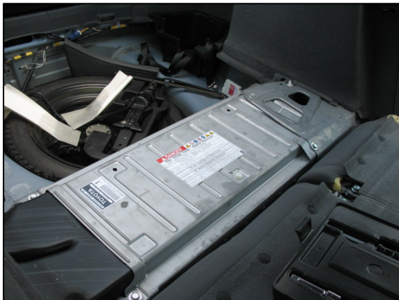
Figure 8: Toyota hybrid battery with aluminum cover in place.
