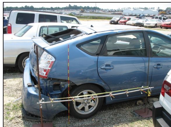
Figure 5: Initial impact damage to the Toyota.
