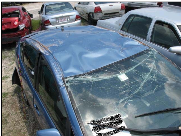
Figure 6: Toyota rollover damage from above, right front.
