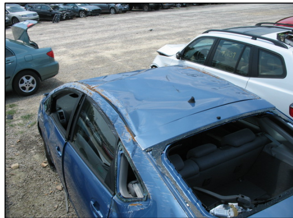
Figure 7: Toyota rollover damage from above, left rear.
