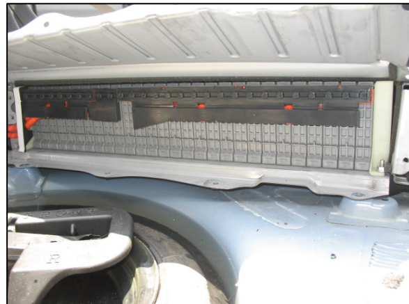
Figure 9: Individual cells of Toyota hybrid battery with cover elevated.
