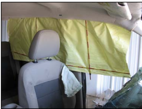
Figure 9: Left curtain air bag.
