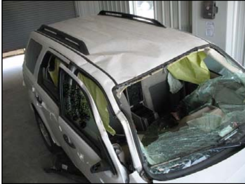
Figure 6: Rollover damage from above, right front.
