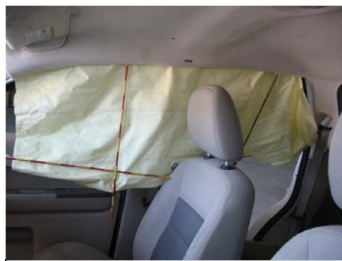
Figure 10: Right curtain air bag.
