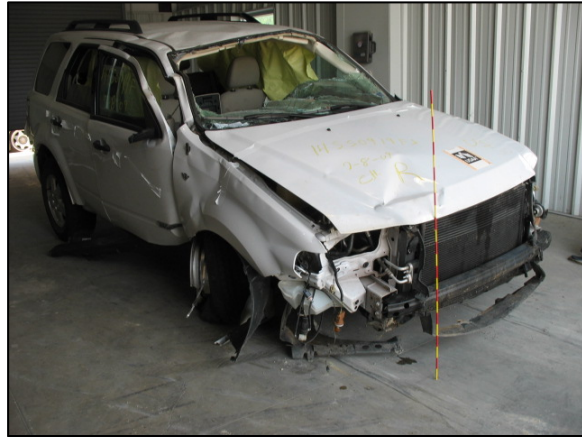
Figure 5: Initial impact damage to the Ford.
