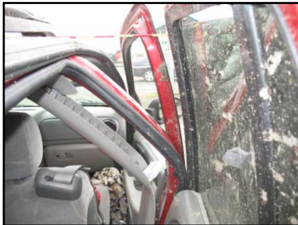
Figure 7: View of the maximum deformation at the right B-pillar location.
