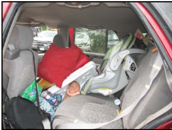
Figure 9: Overall view of the second row after removal of the left CRS (displaced cooler, lid and right CRS on the seat cushion).
