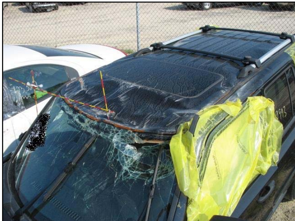
Figure 5: Overall view of the damage to the Jeep's top plane.
