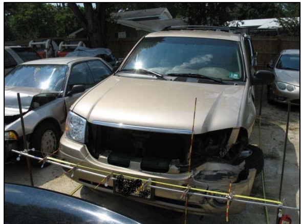
Figure 9: Initial impact damage to the GMC.
