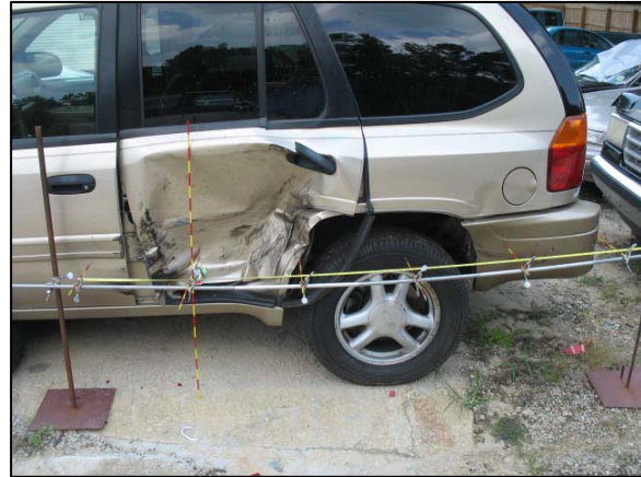
Figure 10: Secondary impact damage to the left side of the GMC.
