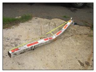
Figure 12: View of the separated rear impact guard beam.
