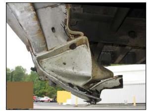
Figure 9: Right side view of the deformed rear impact guard vertical support.
