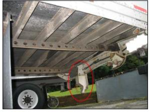
Figure 3: Left view of the trailer depicting the slider frame and the attachment of the rear impact guard.
