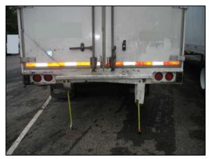
Figure 8: Back view of the trailer and deformed rear impact guard.
