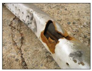
Figure 14: View of the right side of the guard beam and the torn metal surrounding the welded connection of the intermediate plate.
