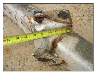
Figure 13: View of the left end of the guard beam and the welded intermediate connection plate.
