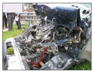
Figure 15: Left view of the frontal deformation. The left body mount is highlighted in the image.
