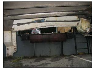
Figure 11: View looking rearward of the deformed back plane and rear impact guard supports.
