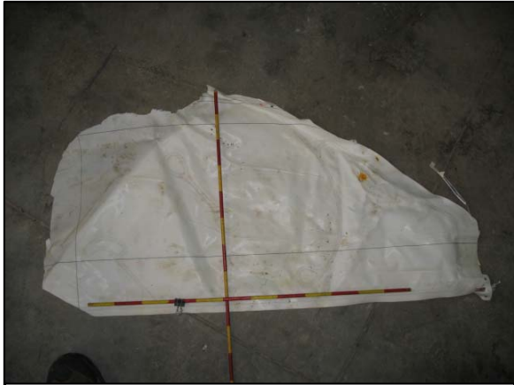
Figure 6: Forward section of left IC cut from the vehicle.
