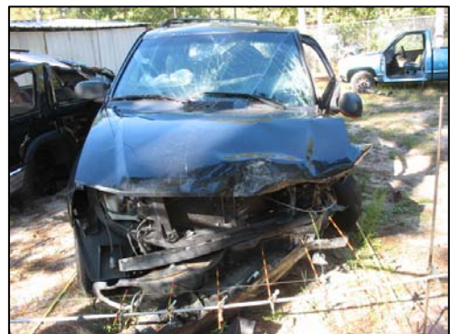
Figure 9: Frontal damage to the Chevrolet.
