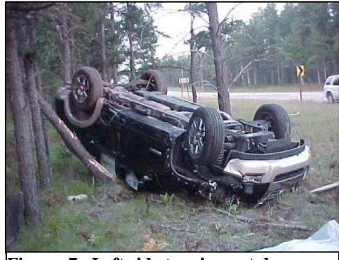
Figure 7. Left side tree impact damage.
