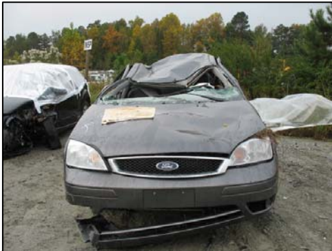
Figure 4: Front bumper fascia damage and roof crush from the front of the Ford.
