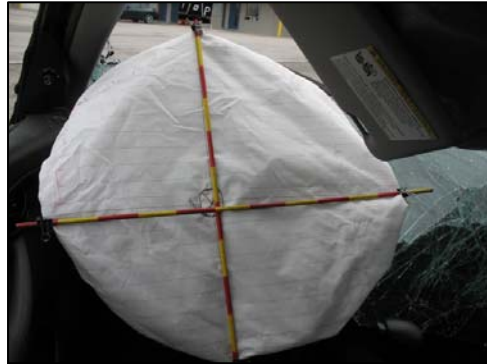
Figure 6: Deployed driver's frontal air bag.
