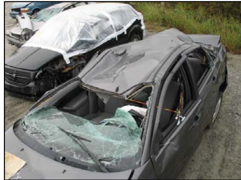
Figure 5: Rollover damage from above, left front.
