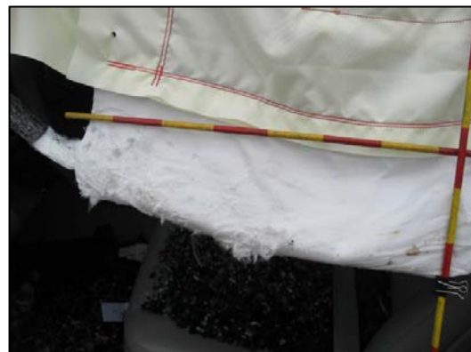
Figure 5: Abrasion to the outer aspect of the left curtain.
