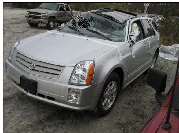
Figure 4: Rollover damage to the left and top planes of the Cadillac.
