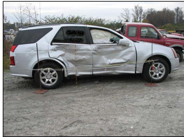
Figure 3: Right side damage to the Cadillac.
