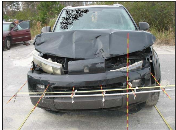
Figure 8: Frontal damage to the Saturn.
