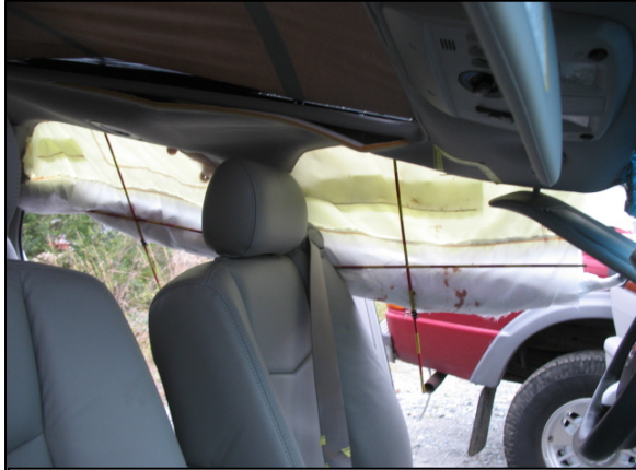
Figure 6: Left IC air bag of the Cadillac SRX.
