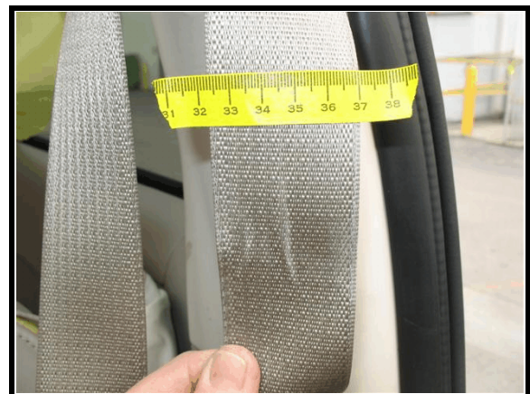
Figure 10. Scuff to driver's safety belt
