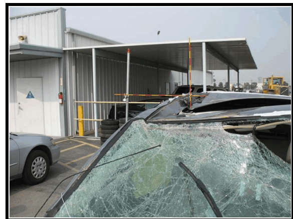
Figure 6. Maximum vertical crush, 2008 Ford Escape
