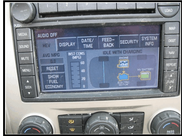
Figure 15. Center IP display. Vehicle running and HV battery being charged.
