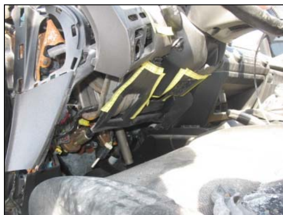
Figure 7: View of the driver's lower extremity contact to the Honda's intruded lower instrument panel.
