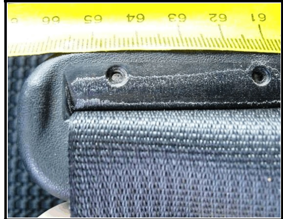
Figure 5. Driver's safety belt latch plate showing scuff marks
