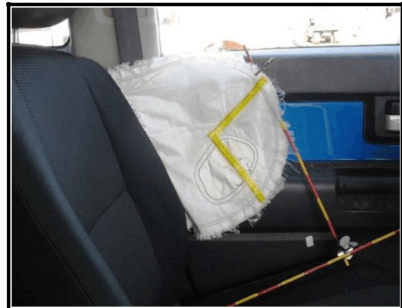
Figure 7. Left seat-mounted side air bag showing location of skin oil transfer
