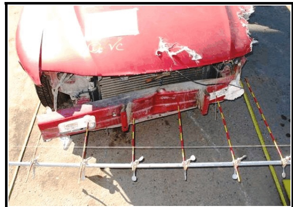
Figure 8. Front end crush profile measurement
