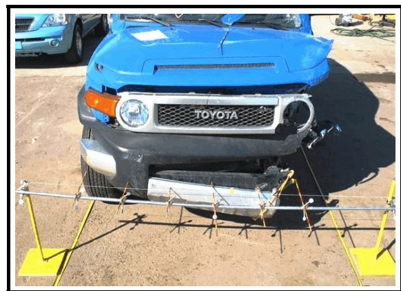
Figure 3. Subject vehicle, front end crush profile measurement
