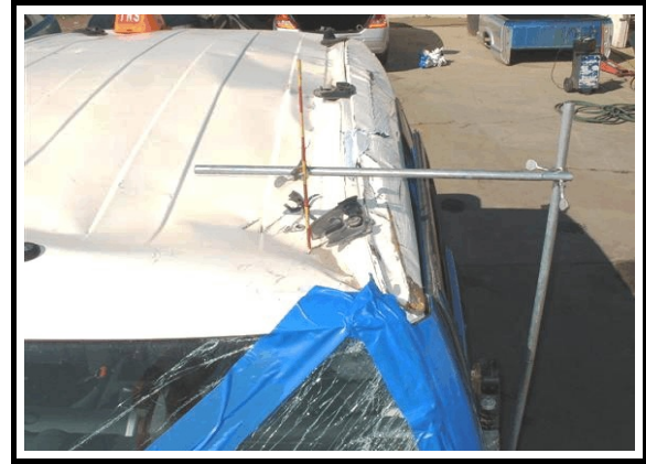
Figure 4. Subject vehicle, maximum vertical roof crush measurement
