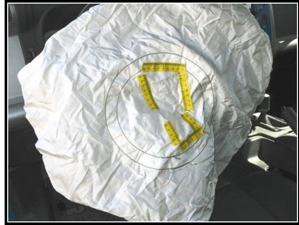
Figure 6. Frontal air bag showing location of occupant loading
