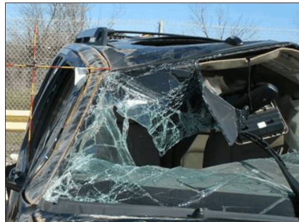
Figure 7: The maximum lateral and vertical crush occurred at the top of the right A-pillar
