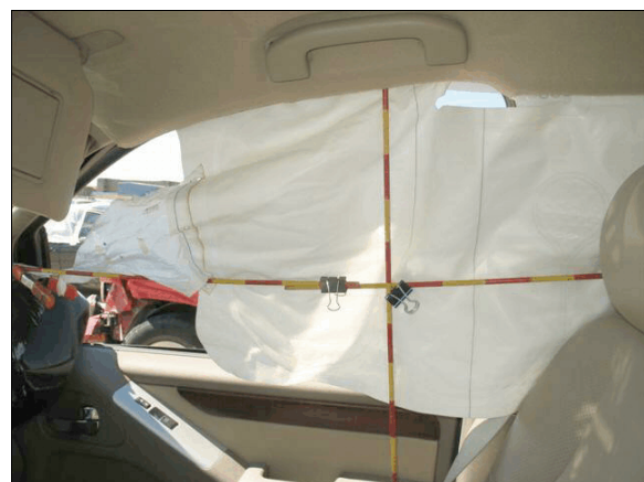
Figure 10: The front of the right IC air bag
