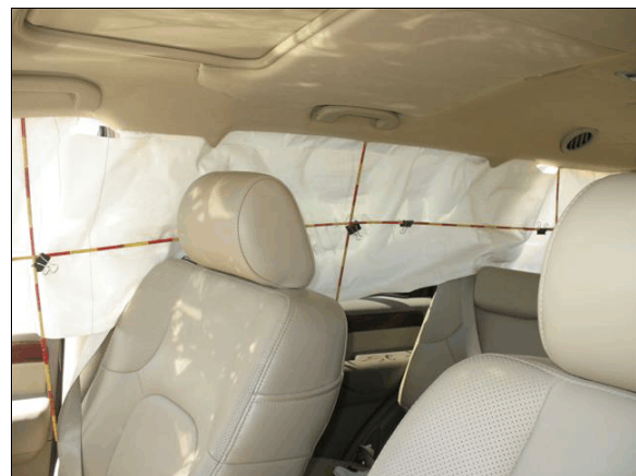
Figure 9: The back portion of the deployed right IC air bag
