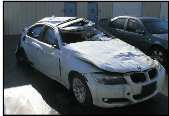
Figure 4. Rollover damage, 2009 BMW 328i
