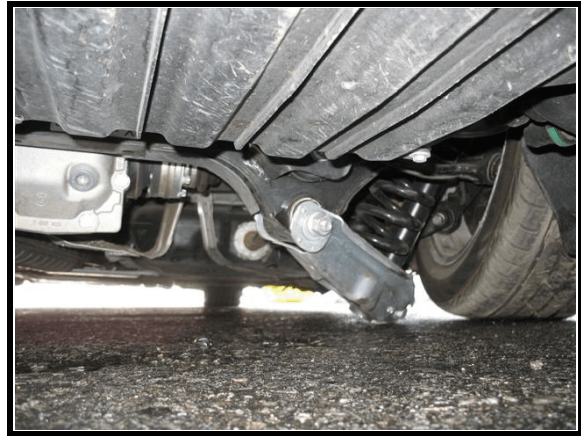
Figure 6. Right rear strut displaced
