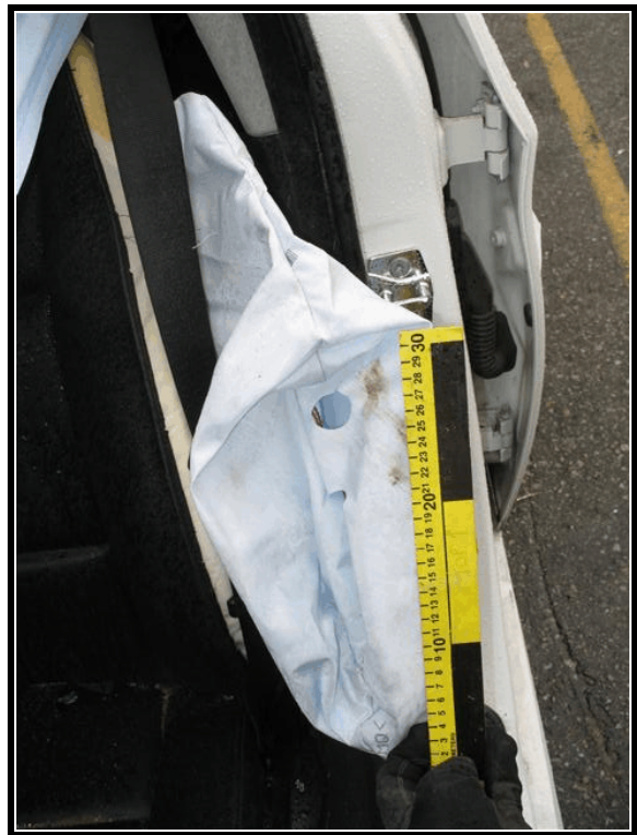
Figure 10. Driver's seat-mounted side air bag
