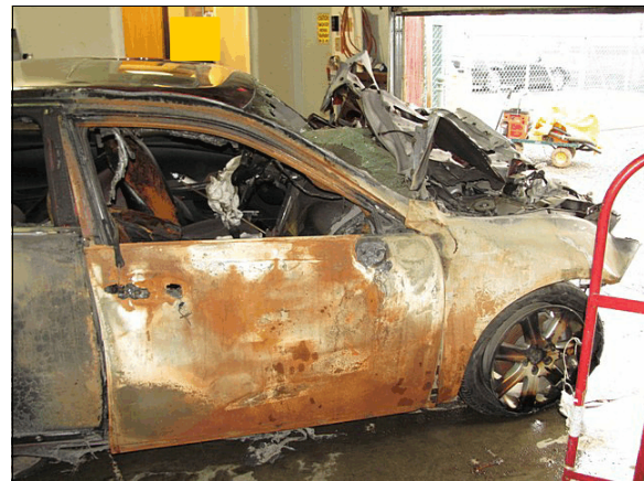
Figure 8: Right side view of the damage on the Lexus from the fire
