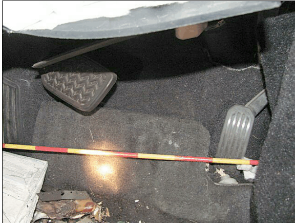
Figure 10: The initial status of the driver's floor mat, accelerator pedal, and brake pedal at the SCI inspection
