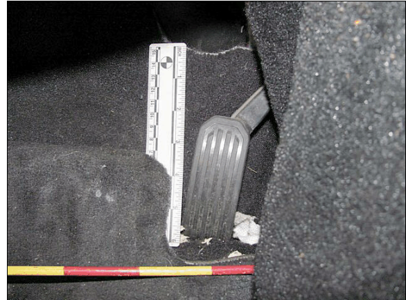
Figure 11: The end of the accelerator pedal was entrapped in a fold in the damaged carpet
