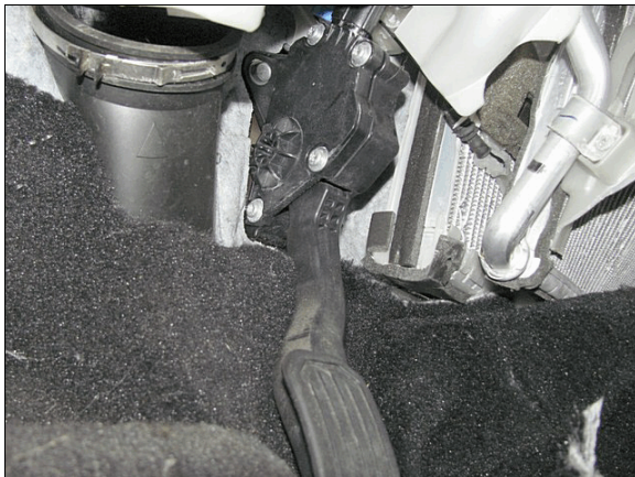
Figure 12: The Denso accelerator mechanism housing
