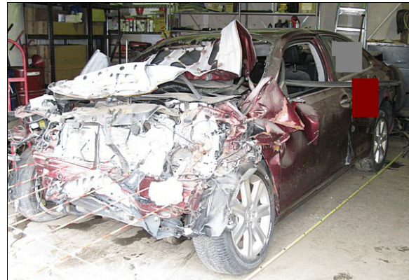
Figure 4: The damage on the front plane of the Lexus from the impact with the front of the Ford
