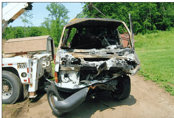
Figure 15: Police photo of the front plane damage on the Ford from the impact with the Lexus
