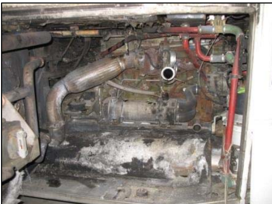
Figure 14. Muffler heat shield damage.
