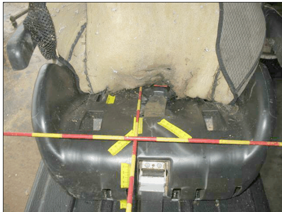
Figure 10: Yellow tape highlights crack and stress marks in shell of CRS
