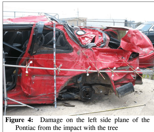
Figure 4: Damage on the left side plane of the Pontiac from the impact with the tree
