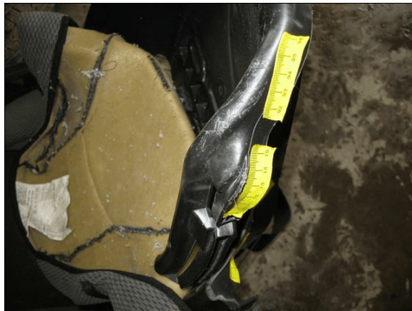
Figure 12: Abrasions on the top left portion of the shell of the CRS
