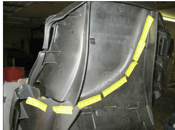
Figure 11: Crack and stress mark on upper left portion of the shell of the CRS
