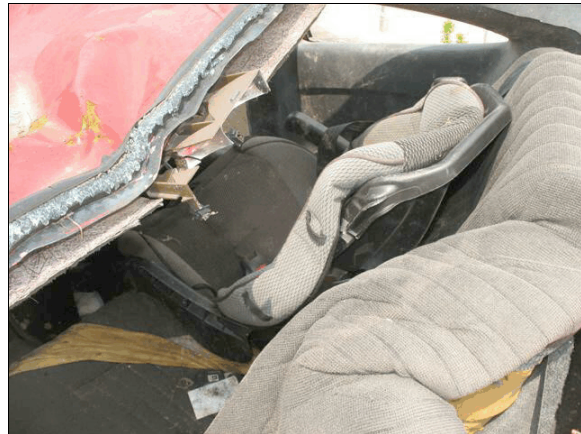
Figure 8: The CRS was found secured in the second row right seating position of the Pontiac at the SCI inspection
