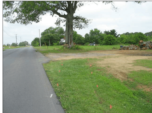
Figure 3: Approach to impact with the tree; orange flags show yaw marks in the grass; yaw mark on left is left rear tire; yaw mark on right is left front tire
