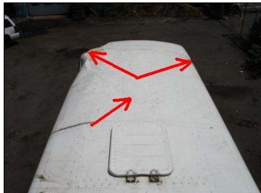
**Figure 12: Roof damage from towing activities.**
