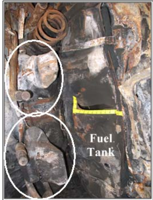
Figure 13: View of the damaged fuel tank and deployed FSS (circled).
