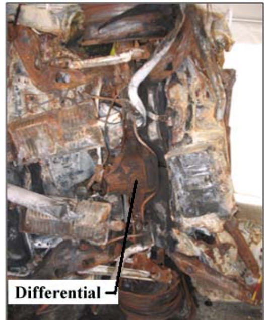
Figure 12: Close-up view of the damaged rear undercarriage of the Ford prior to disassembly.
