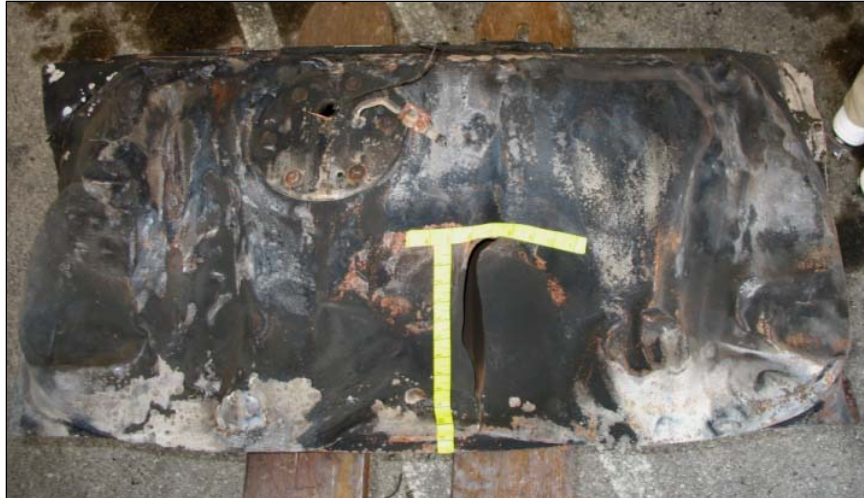
Figure 15: View of the forward wall of the removed fuel tank and the large split/tear.
