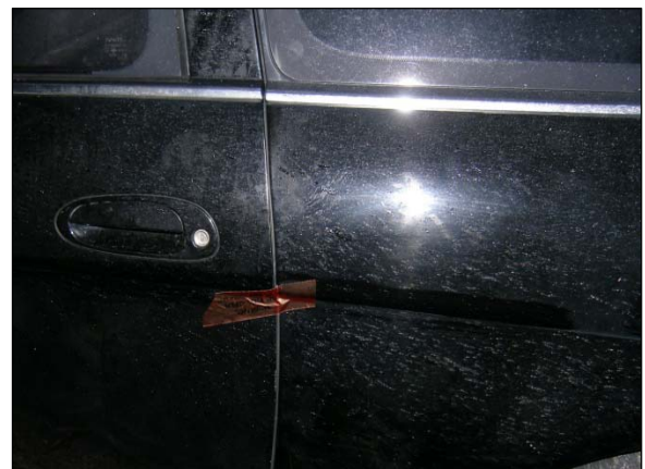
Figure 18: AFFF suppressant/surfactant residue on the exterior surfaces of the Lexus.
