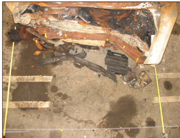
Figure 9: Overhead view of the damage profile to the back plane of the Ford.
