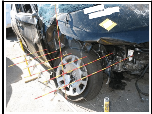
Figure 4. Right side crush measurement, 2010 Scion xD
