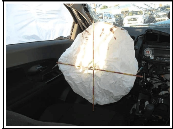
Figure 7. Driver's deployed frontal air bag, 2010 Scion xD
