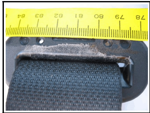
Figure 6. Driver's safety belt showing load marks, 2010 Scion xD
