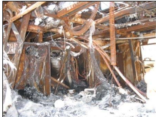
Figure 11. View from the right rear luggage bay looking rearward at the electrical boxes and the AC system components.
