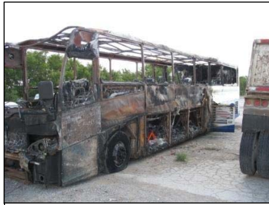
Figure 7. Left side view of the fire damage to the MCI motorcoach.
