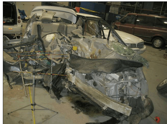
Figure 4: Damage on the front and right side planes of the Prius from the impact with the Chevrolet; crush measurement were documented on both front and side planes
