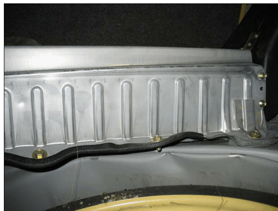
Figure 7: Minor deformation of the mounting flange on the back of the Toyota's propulsion battery
