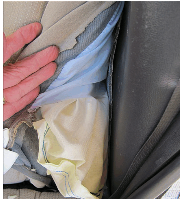
Figure 10: The partially unfolded condition of the driver's seat-mounted side impact air bag
