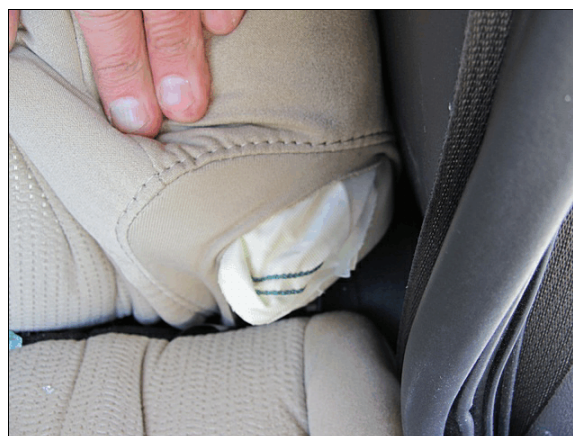
Figure 9: Small portion of the driver's seat mounted side impact air bag was protruding out of the bottom of the seat back
