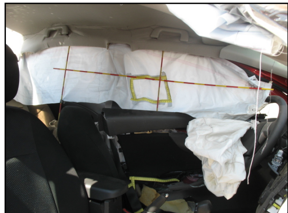
Figure 10: Inboard side of left IC air bag, including driver's head contact.
