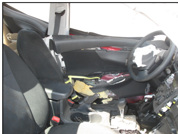
Figure 8: Deformation of the front left seat as a result of intrusion.
