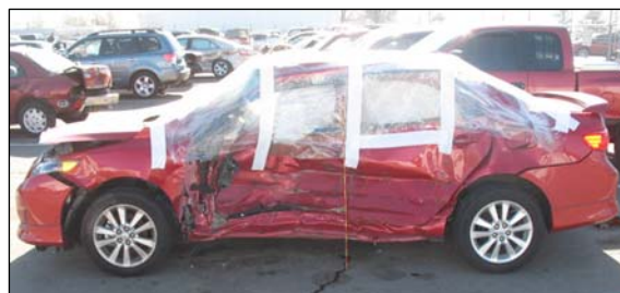
Figure 6: Event 1 impact damage to the left side of the Toyota.
