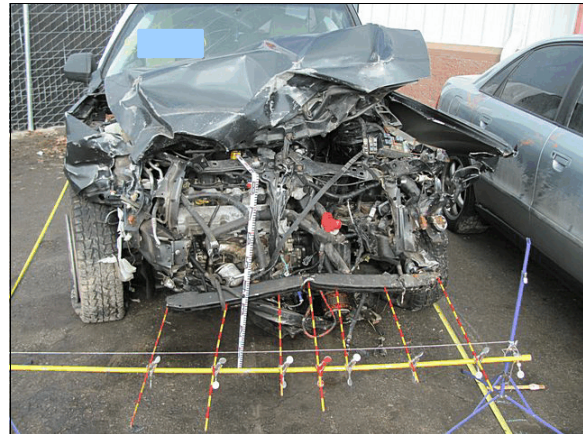
Figure 4: Damage to the front plane of the Ford from impact with the Toyota
