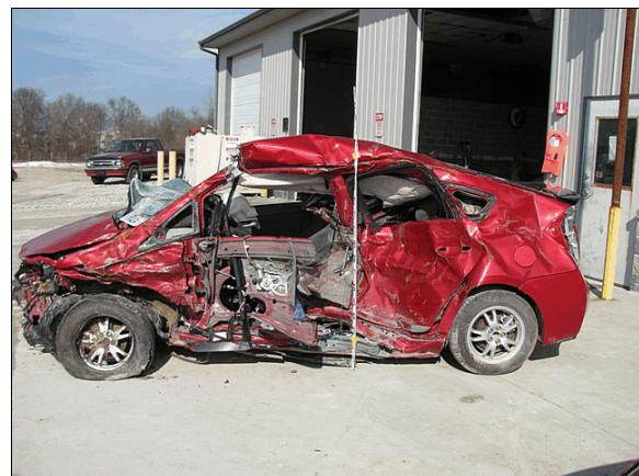
Figure 5: Damage on the left plane of the Toyota from the impact with the Ford
