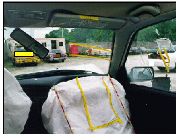
Figure 11: Case vehicle's deployed front right air bag showing occupant contact evidence to upper center portion of air bag, sun visor, and right front glazing (case photo #44)
