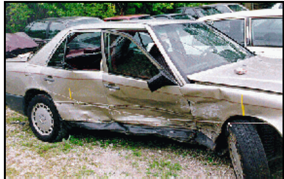
Figure 16: Mercedes Benz's right side damage viewed from right of front; Note: yellow tape marks width of direct contact (case photo #61)
