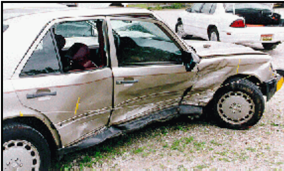
Figure 15: Mercedes Benz's right side damage view-ed from back of right; Note: vertical yellow tape marks width of direct damage (case photo #59)
