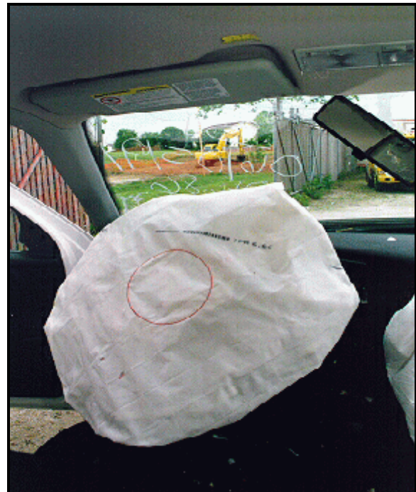
Figure 10: Case vehicle's deployed driver air bag showing no clear evidence of driver contact (case photo #28)
