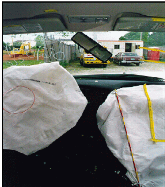
Figure 9: Case vehicle's deployed air bags viewed from back seat; Note: rear view mirror knocked askew by front right air bag (case photo #34)
