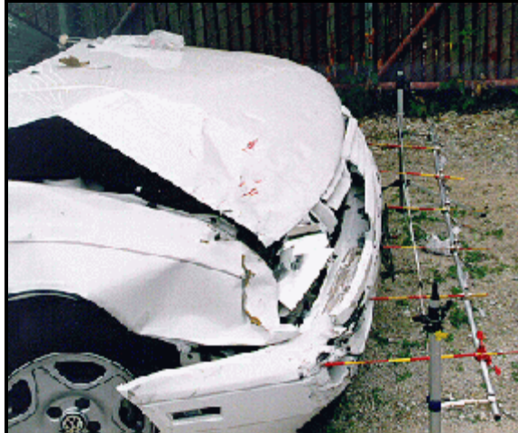
Figure 14: Reference line view of case vehicle's frontal damage from right; Note: crush primarily to front right corner (case photo #22)
