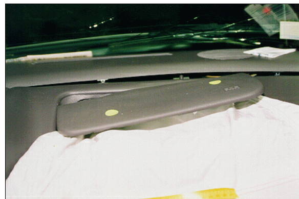
Figure 6: Close-up view of case vehicle's misaligned front right air bag module's cover flap, indicating the air bag's deployment path was momentarily altered/blocked (case photo #47)
