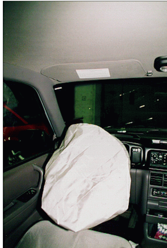
Figure 5: Vertical view of case vehicle's driver seating area; Note: no visible evidence of contact to driver's air bag (case photo #30)
