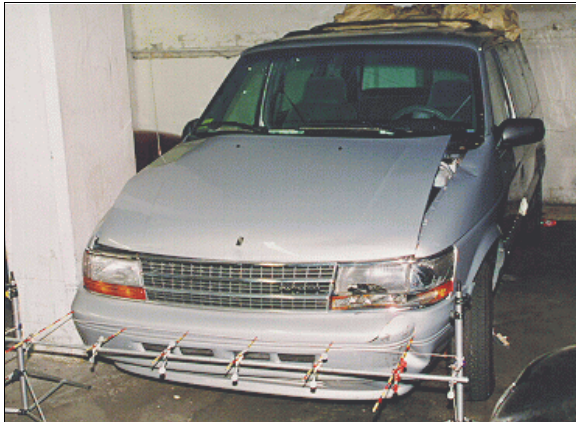
Figure 3: Case vehicle's frontal damage with contour gauge present viewed from left of center; Note: front end shifted slightly to right (case photo #16)
