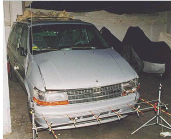
Figure 4: Case vehicle's frontal damage with contour gauge present viewed from right of center; Note: front end shifted to right (case photo #27)
