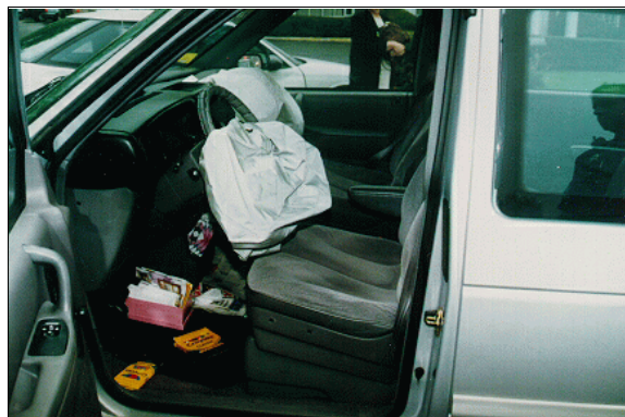
Figure 14: On-scene view of case vehicle's front seating area showing deployed front air bags and driver's seat track location (case photo #33)
