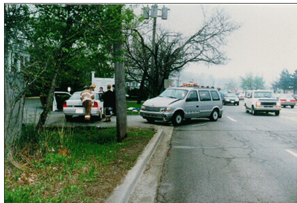
Figure 1: On-scene view of case vehicle (diagonally straddling outside lane) and Oldsmobile (toward left) at final rest positions; Note: both vehicles rotated clockwise post-impact (case photo #05)
