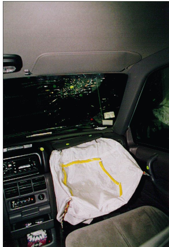
Figure 2: Vertical view of case vehicle's front right seating area showing contact evidence to top of front right passenger air bag, right side of center instrument panel, and cover flap (yellow dots); Note: windshield contacted by deploying air bag (case photo #38)
