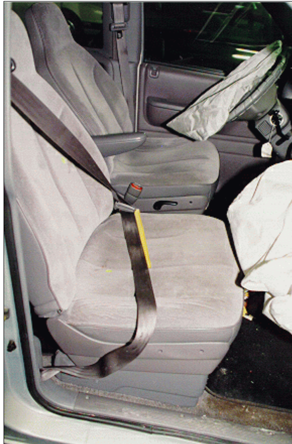
Figure 13: Case vehicle's front right seat belt showing area of blood smear (taped area) and blood spots (yellow dots) to seat cushion and seat back (case photo #34A)
