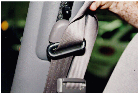
Figure 9: Close-up of "D"-ring from case vehicle's front right passenger seat belt showing heat abrasion indicating some type of usage during crash (case photo #60A)
