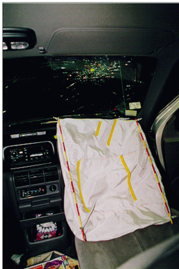
Figure 7: Vertical view of case vehicle's front right passenger seating area and deployed front right air bag; Note: skin evidence on front portion of air bag, highlighted by yellow tape (case photo #42)
