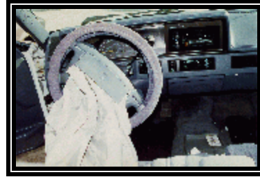
Figure 4. Upper module cover flap and the deployed air bag
