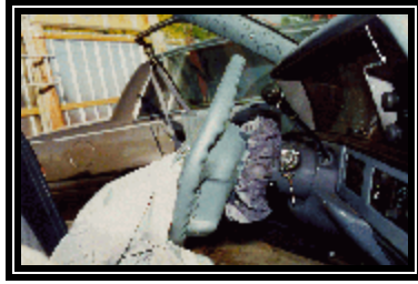
Figure 3. Perpendicular view of the deployed air bag and the steering wheel rim
