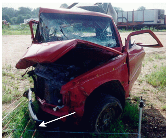
Figure 6: 1st other vehicle's front right damage showing severe rightward shift of front end; Note: position of C1 (case photo #51)
