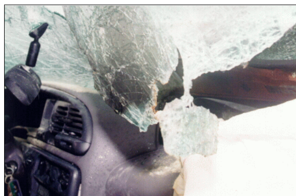
Figure 20: Close-up of case vehicle’s holed windshield showing blood on edge of broken glazing (case photo #32)
