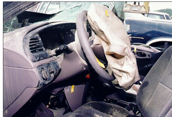
Figure 22: Case vehicle's driver seating area showing deployed driver air bag and distorted driver's seat back; Note: seat back was rotated counterclockwise from contact by back left passenger (case photo #39)
