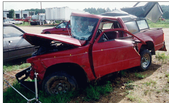
Figure 23: Sideswipe damage along 1st other vehicle's left side from impact with 2nd other vehicle's left side (case photo #53)
