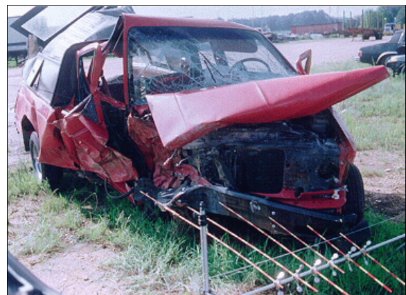
Figure 7: 1st other vehicle's front right damage, viewed from right of front, with contour gauge present showing offset nature of impact (case photo #64)
