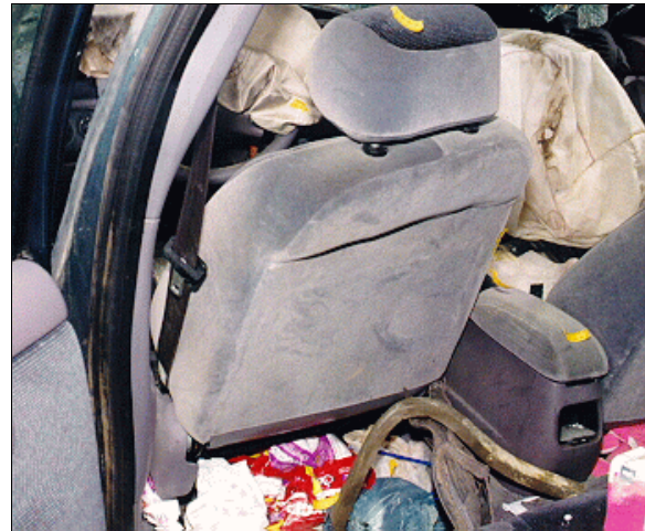
Figure 15: Back of case vehicle's driver seat showing occupant contact evidence on top of head restraint and back of center console (case photo #44)
