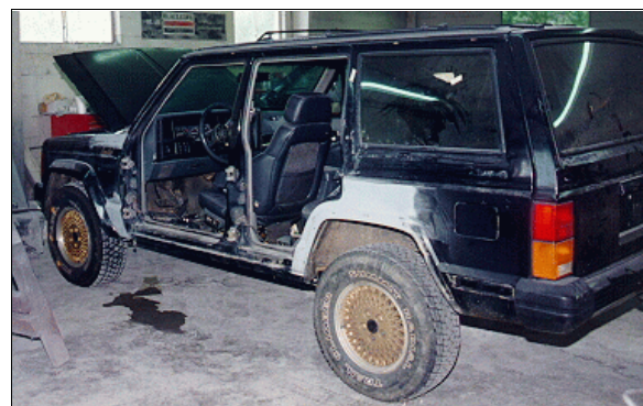
Figure 24: Left side of 2nd other vehicle, viewed from left of back; showing repairs in progress resulting from sideswiping impact by front left of 1st other vehicle (case photo #69)
