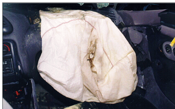
Figure 18: Case vehicle's deployed front right passenger air bag showing holed and burned area of fabric in center of air bag (case photo #40)
