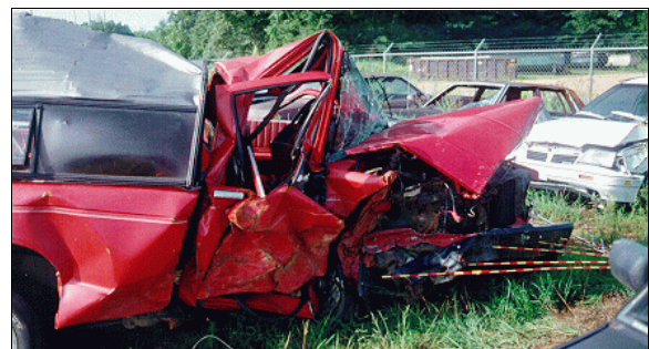
Figure 8: 1st other vehicle's right side showing right front tire which was shoved backwards under-neath damaged right "A"-pillar; Note: roof buck-ling (case photo #62)
