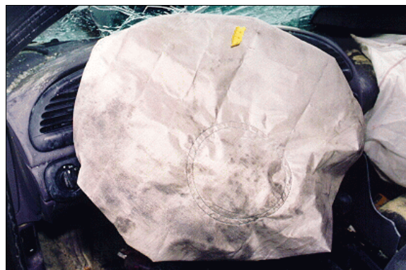
Figure 17: Case vehicle's deployed driver air bag showing contact evidence on bag's fabric near 12 o'clock position (case photo #37)
