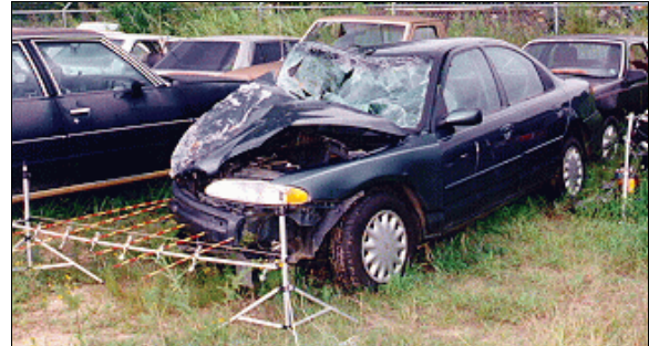
Figure 5: Case vehicle's front right damage viewed from left of front with contour gauge present showing offset nature of impact (case photo #13)
