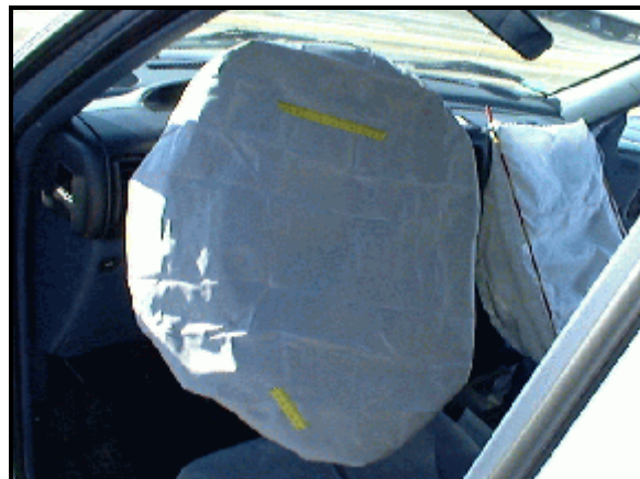
Figure 8: Case vehicle's driver air bag with tape indicating areas of skin and cloth transfer; Note: steering wheel rotated approximately 90 degrees counterclockwise (case photo #21)
