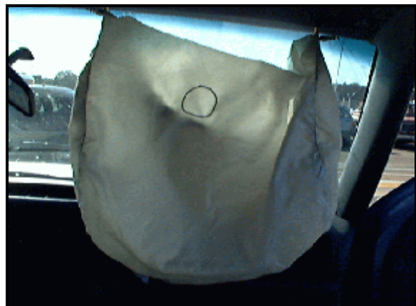
Figure 10: Underside (bottom) of case vehicle's front right passenger air bag showing area of skin transfer (circled area) from front right passenger's face (case photo #33)
