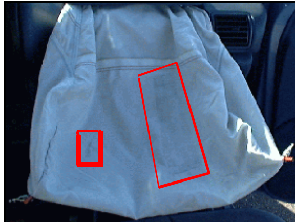
Figure 15: Top surface of case vehicle's front right air bag showing no contact from front right passenger, but contact evidence is present from rearview mirror (small highlight) and cover flap transfer (large highlight) (case photo #31)
