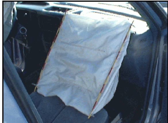
Figure 9: Front surface of case vehicle's front right passenger air bag showing no evidence of contact (case photo #29)
