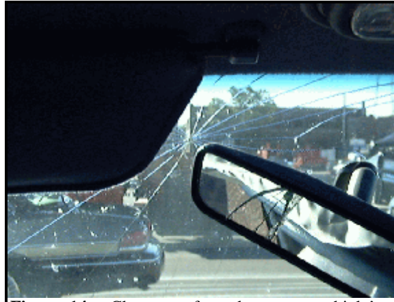
Figure 14: Close-up of crack to case vehicle's windshield caused by contact from rearview mirror (case photo #47)
