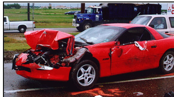
Figure 2: On-scene view of case vehicle at final rest; Note: underride type damage to front and swiping type damage to left side (case photo #58)
