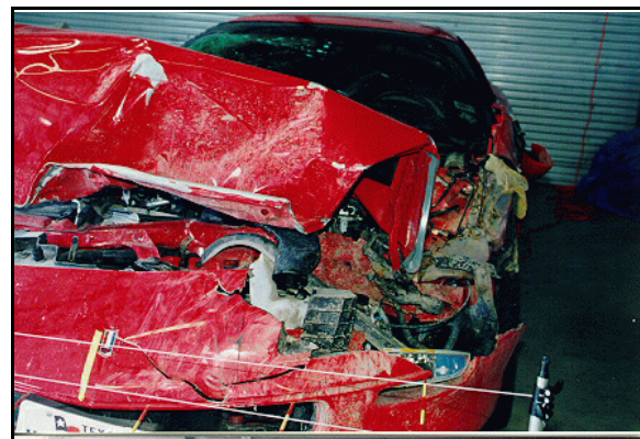
Figure 3: Close-up showing direct damage width to case vehicle's front left bumper (case photo #14)
