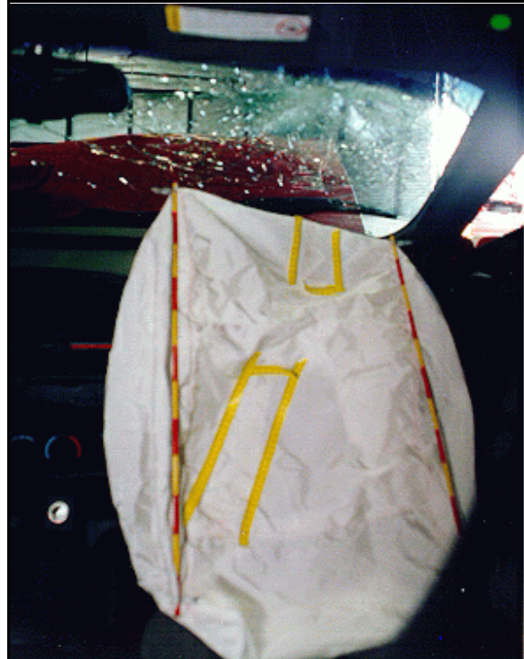
Figure 7: Vertical view of case vehicle's front right passenger air bag showing skin transfers to air bag; Note: sun visor contact and windshield damaged from cover flap (case photo #33)
