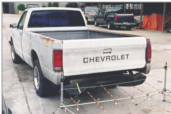
Figure 18: Chevrolet pickup's damaged back with contour gauge present; Note: bumper rotated under truck bed allowing case vehicle to underride (case photo #56)
