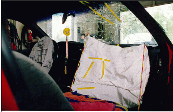
Figure 11: Case vehicle's front right seating area showing deployed front air bags and contact (yellow tape) on deployed front right air bag and windshield's glazing (case photo #50)
