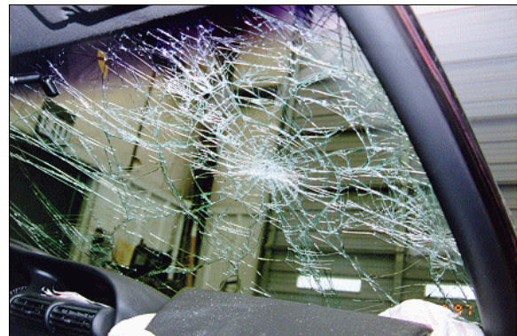
Figure 15: Case vehicle's right windshield glazing showing contacts to glazing and front right header by front right passenger's head (case photo #33a)
