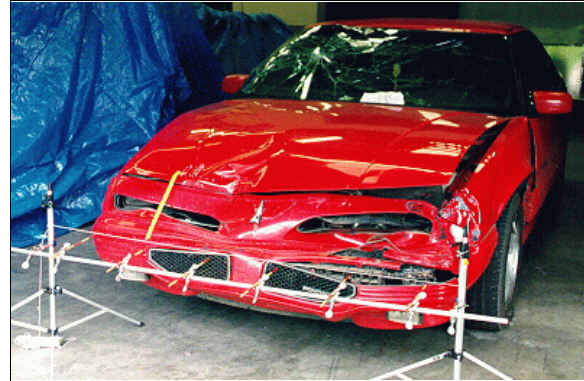
Figure 5: Case vehicle's frontal damage viewed from left of front with contour gauge present; Note: yellow tape indicates end of direct damage width (case photo #12)
