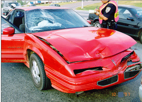
Figure 4: On-scene view of case vehicle at final rest; Note: damage to right half of hood and right windshield's glazing (case photo #09)
