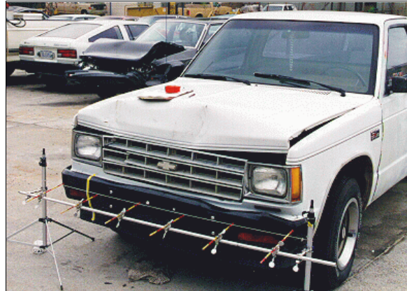
Figure 20: Chevrolet pickup's frontal damage from impacting back of Chevrolet van; Note: yellow tape indicates end of direct damage (case photo #64)
