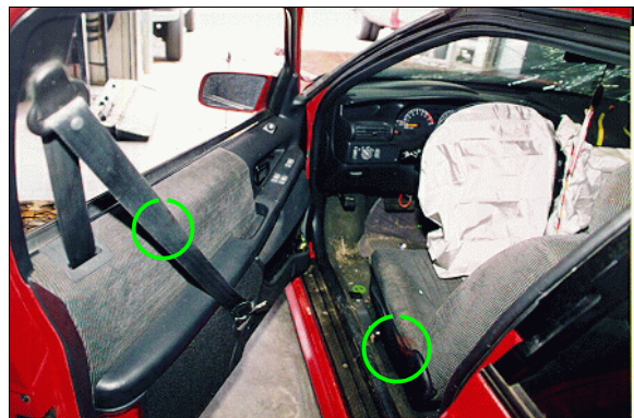
Figure 10: Interior view of case vehicle’s driver seating area showing blood transfers on webbing of driver’s automatic seat belt and on left side of seat cushion (Case Photo #21)
