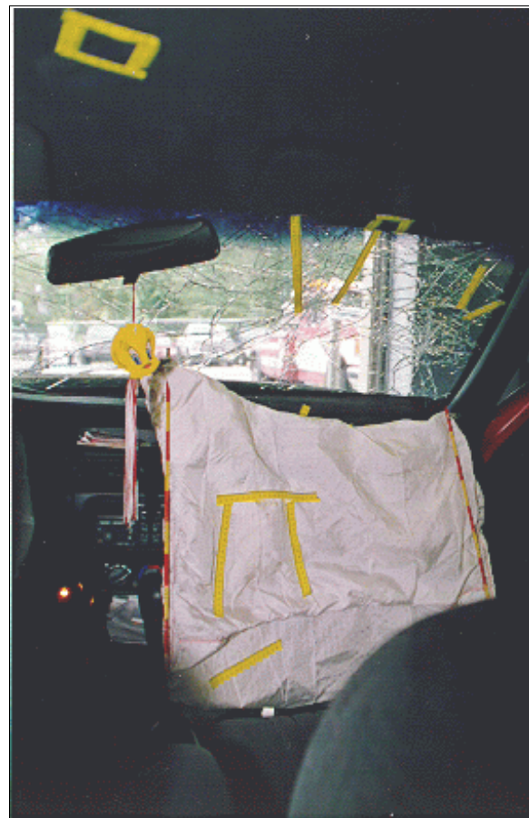
Figure 8: Vertical view of case vehicle's front right passenger seating area showing contact (i.e., yellow tape) areas on deployed air bag, windshield's glazing, front right header, and roof (case photo #34)
