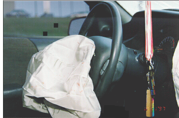
Figure 12: Case vehicle's deployed driver air bag showing black cover flap transfers and blood splatter on part of air bag's front surface (case photo #30)
