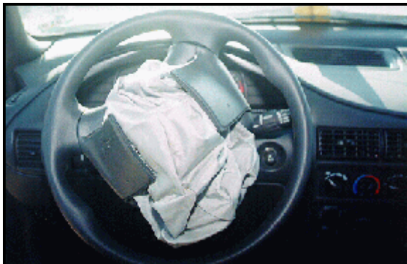
Figure 11: Case vehicle's deployed driver air bag showing "I"-type cover flaps without evidence of damage or occupant contact (case photo #25)
