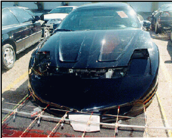
Figure 6: Vehicle #2's frontal damage with contour gauge present at bumper level; Note: damage was primarily to front right corner (case photo #36)
