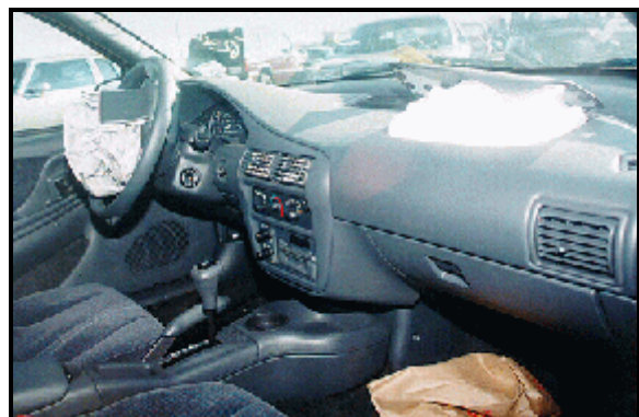
Figure 10: Case vehicle's front seating area showing deployed driver and front right air bags and floor-mounted automatic transmission (case photo #28)
