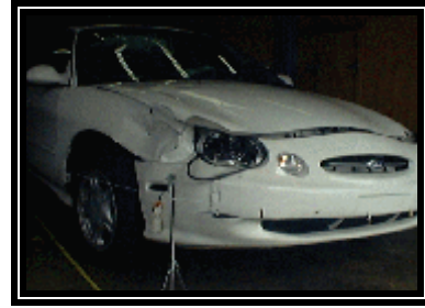
Figure 4. Initial front right corner impact damage to the Ford Taurus.
