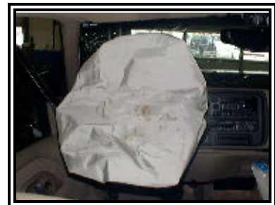
Figure 6: Driver air bag.
