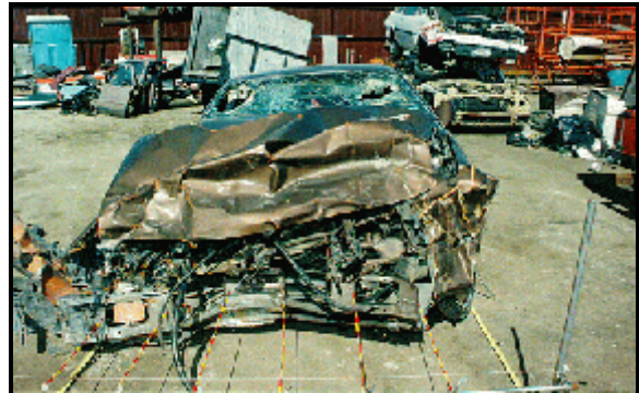
Figure 7: Vehicle #2's frontal damage with contour gauge present from initial impact with case vehicle (case photo #47)
