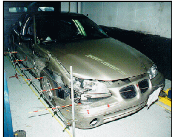
Figure 3: Case vehicle's right side damage with contour gauge present viewed from left of front (case photo #14)
