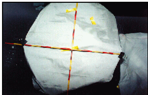
Figure 13: Case vehicle's deployed driver air bag; Note: yellow tape identifies possible contact points (case photo #29)
