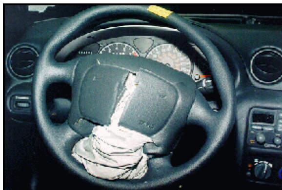
Figure 12: Case vehicle's steering wheel-mounted driver air bag module showing "I" configuration cover flaps without evidence of damage or occupant contact (case photo #33)
