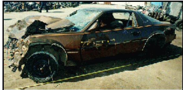
Figure 10: Vehicle #2's driver door damaged from sideslap impact with case vehicle (case photo #51)
