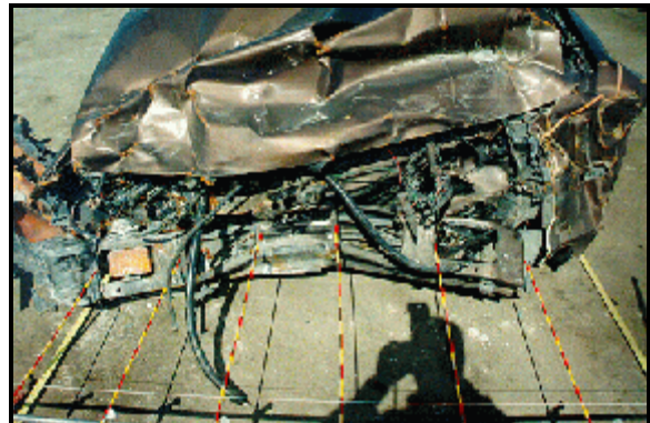
Figure 8: Close-up of vehicle #2's frontal damage with contour gauge present (case photo #48)
