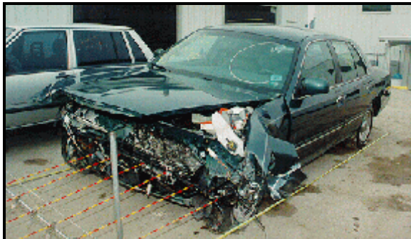
Figure 6: Vehicle #2's frontal damage from impact with case vehicle’s left side viewed from left of front with contour gauge present (case photo #43)
