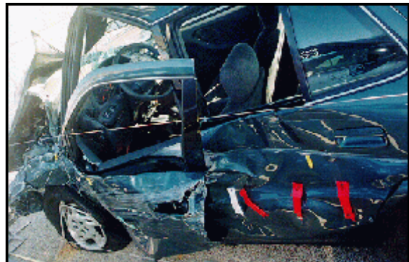
Figure 5: Damage along case vehicle’s left side from impact with vehicle #2 viewed from left back (case photo #16)
