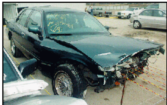
Figure 7: Vehicle #2's frontal damage from impact with case vehicle’s left side viewed from right of front with contour gauge present (case photo #49)
