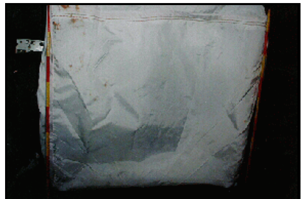
Figure 14: Case vehicle's deployed front right air bag; Note: blood on upper left quadrant is from driver's head lesions as he lay against air bag at final rest (case photo #50)
