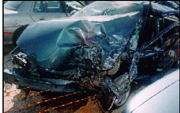
Figure 4: Case vehicle’s overlapping front left and left front damage from deployment impact with vehicle #2 and front left damage from impact with signal pole; Note: contour gauge is present for signal pole impact (case photo #13)
