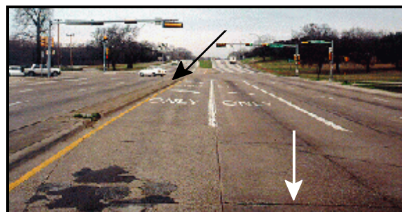
Figure 3: Vehicle #2's travel path, similar to white car above, began in outside left-hand turn lane (white arrow) of westbound roadway, prior to left-hand turn across eastbound roadway at four-leg intersection; Note: black arrow marks approximate point of impact (case photo #08)
