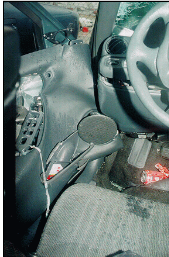
Figure 15: Vertical view of intrusion from driver's door, toe pan, left "A"-pillar, left side panel forward of the "A"-pillar, and left instrument panel into case vehicle's driver seating area; Note: intrusion primarily resulting from impact with vehicle #2 (case photo #24)
